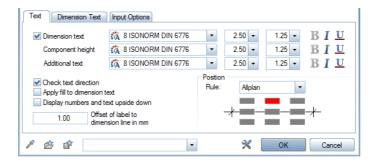
8 Open the **Dimension Text** tab and check the following parameters:
