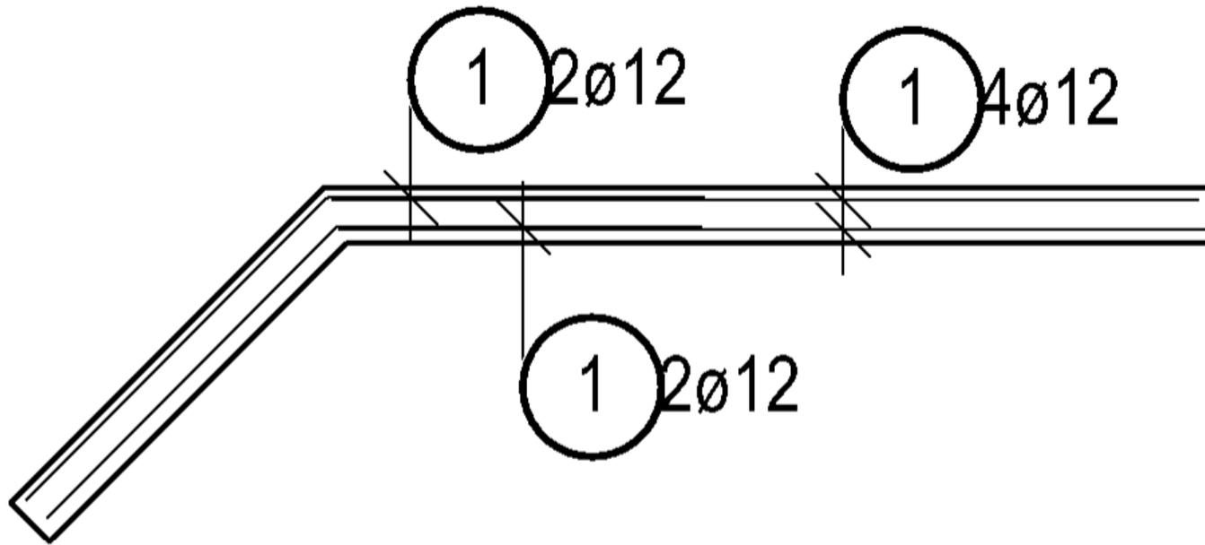
$1 \text{ } \phi 12 / L_{fdM} = 32.91\text{m}$
