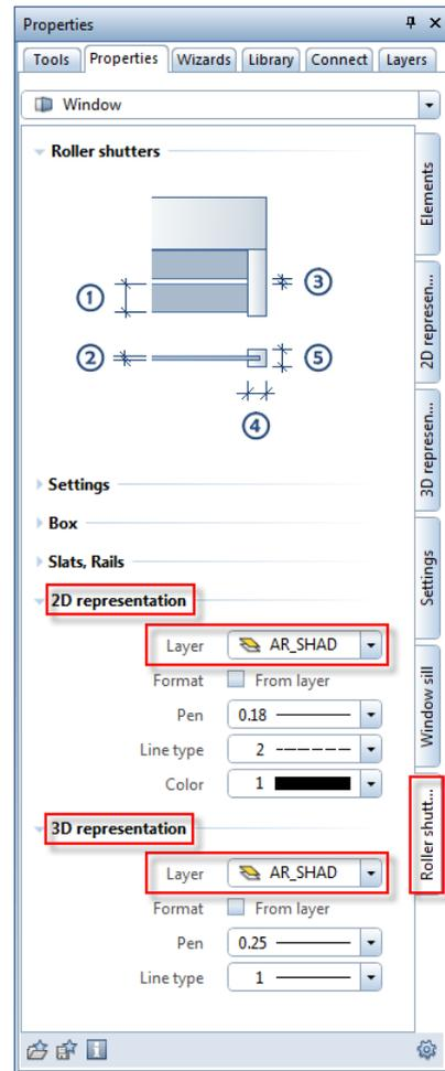
In addition, you can assign different layers when you create separate SmartParts for window sills and roller shutters.
