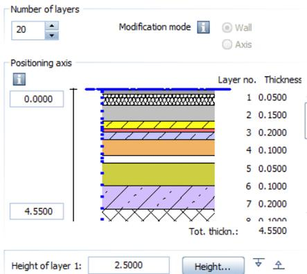
**Important:** in earlier versions, walls could only have up to five layers. If you convert a wall with more than five layers to an earlier version, you get a 3D box for each layer. The geometry of the wall stays the same. Surface elements become 2D surface elements.
