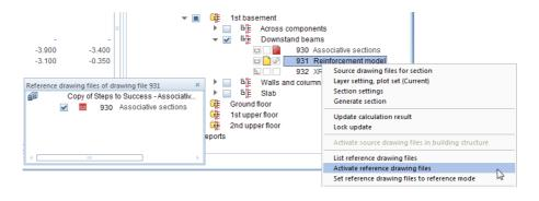
Note: If you want to modify views and sections and the drawing files with the relevant model data are not open in edit mode, the program will issue a message you can use to open the required drawing files in edit mode.
