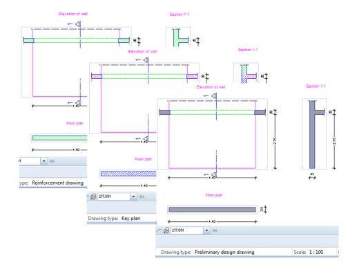
Finally, set the drawing type to **Scale definition** so that the area styles change with the scale.
