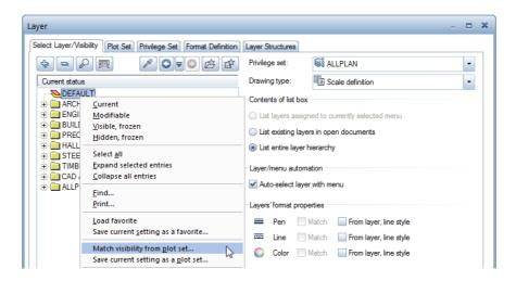
If you have already defined plot sets, you can use them as a basis for additional plot sets. For example, turning the Reinforcement, bottom layer plot set into the Reinforcement, top layer plot set only takes a few mouse clicks.
