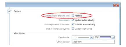
Note: Although you can no longer switch off this option in future Allplan versions, drawing file references are not created as long as all data is in one drawing file.
