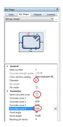
9 The Expand to adapt to edges and Label options are active in the input options. Move the crosshairs in section A-A to the component line on the left within the outline until the bending shape expands, then click in the workspace.
