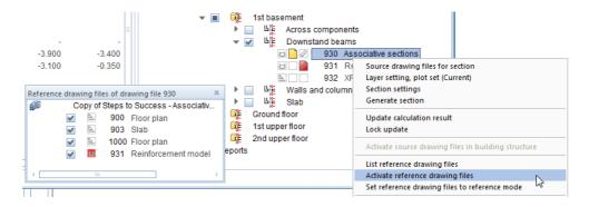
4 To change the reinforcement in the existing views and sections or to add reinforcement, open the dialog box for selecting drawing files. In the "Derived from building structure" area, right-click the drawing file with the reinforcement model: 931 in this example.
